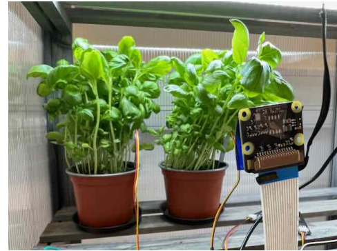
Figure 2: A mini-greenhouse with basil plants and sensors.
